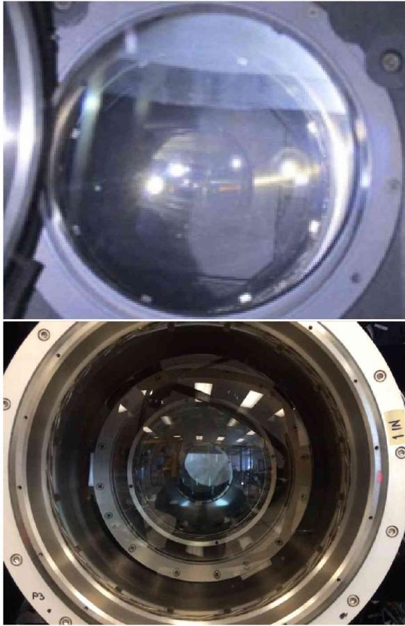
Figure 1: Top: Bubbles in collimator lens group 3 before the intervention. Bottom: Collimator after the oil refill (as seen from lens group 1). Bubbles are gone.
