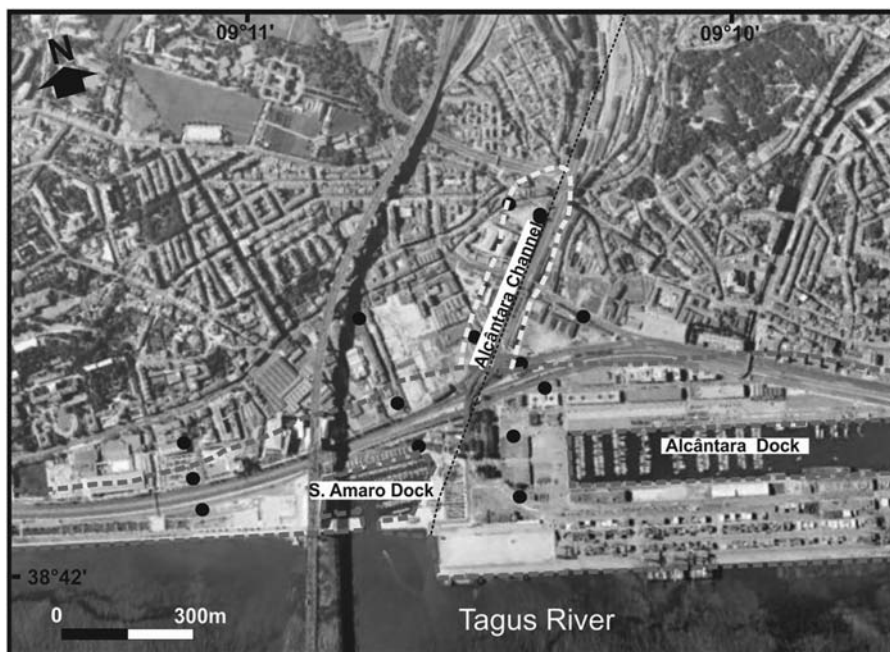
Figure 9 | Location of area of tidal influence and of the salt wedge. The dotted lines bordering the Tagus River, Alcântara Dock and stretching a few hundred metres inland indicates the area with saltwater intrusion. The dotted line surrounding the Alcântara Channel indicates the area of fresh water with strong tidal oscillation. (Full colour version available online.)
