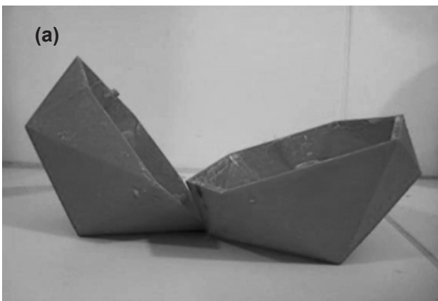
Figure 5: Plastic parts that make up the regular icosahedron made with the 3D printer. Plaster mold of each section to form the icosahedron, for its reproduction on clay.
