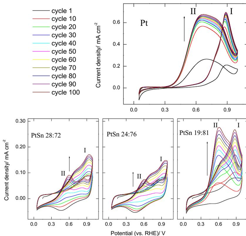
**Fig. 4** Illustrative cyclic voltammograms obtained during 500 cycles of glycerol electrooxidation ( $1.0 \text{ mol L}^{-1}$ ) on Pt and PtSn catalysts.  $\nu = 0.05 \text{ V s}^{-1}$
