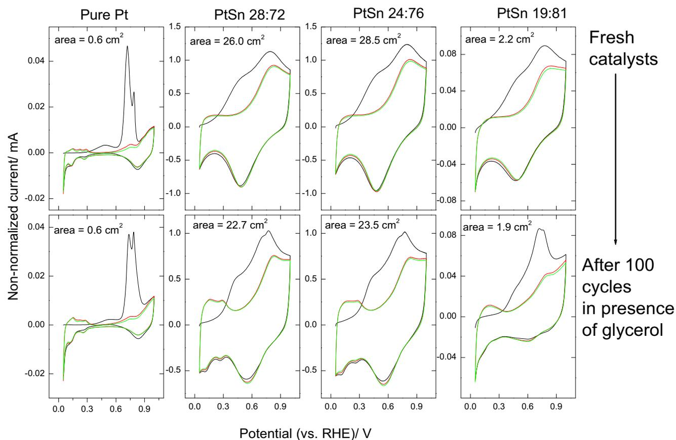
**Fig. 5** CO stripping voltammetry performed on fresh Pt and PtSn catalysts (*top panels*) and after they were submitted to 100 voltammetric cycles in presence of  $1.0 \text{ mol L}^{-1}$  glycerol (*bottom panels*).  $v = 0.02 \text{ V s}^{-1}$
