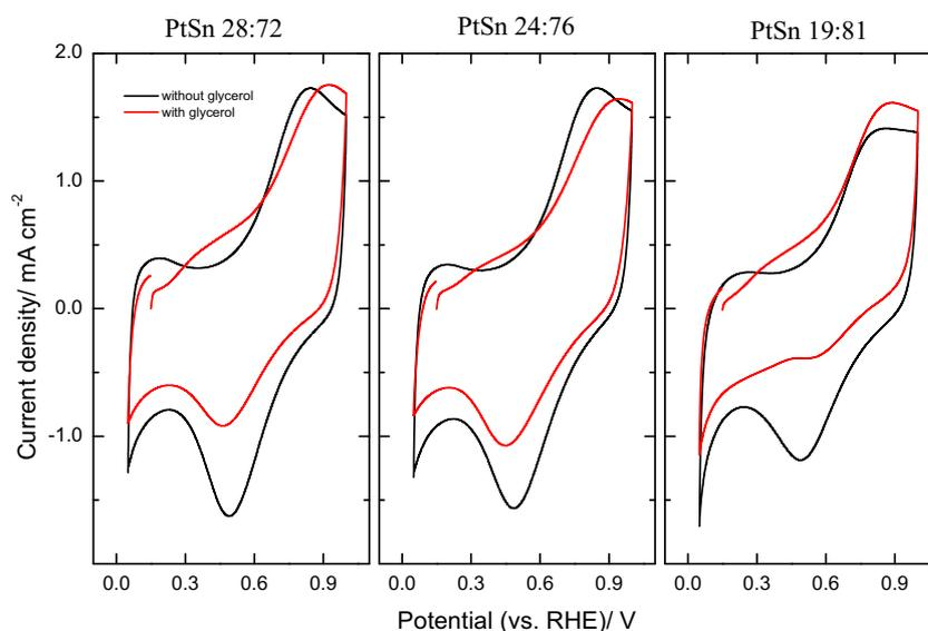
**Fig. 3** Illustrative cyclic voltammograms obtained during 100 cycles of glycerol electrooxidation ( $1.0 \text{ mol L}^{-1}$ ) on Pt and PtSn catalysts.  $\nu = 0.05 \text{ V s}^{-1}$
