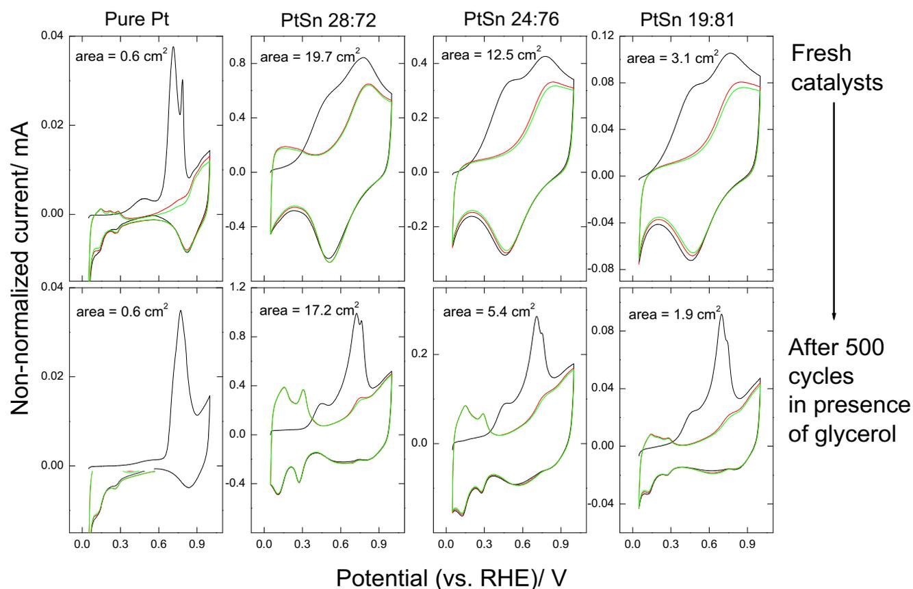
**Fig. 6** CO stripping voltammetry performed on fresh Pt and PtSn catalysts (*top panels*) and after they were submitted to 500 voltammetric cycles in presence of  $1.0 \text{ mol L}^{-1}$  glycerol (*bottom panels*).  $v = 0.02 \text{ V s}^{-1}$
