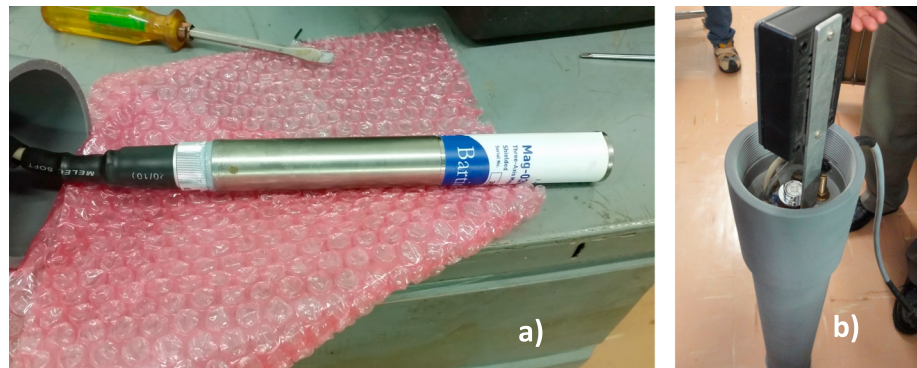
Figure 1. Picture of (a) the single bar sensor core that is built inside (b) the sealed magnetometer sensors PVC enclosure, which composes the Embrace MagNet magnetometer system.
