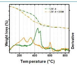
**Figure 7.** Weight loss profile and its corresponding derivative for ZIF-8 nanocrystals and DDM-functionalized ZIF-8. Earlier weight loss between 200 and 300  $^{\circ}$ C points toward the presence of DDM, which is not present in ZIF-8 thermograms.
