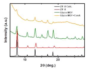
**Figure 6.** X-ray diffractograms obtained for the as-prepared material, DDM-functionalized (Glyco-MOF), and Con A-assembled supraparticles (Glyco-MOF + Con A). In all cases, structures can be safely assumed to retain ZIF-8 characteristic reflections and thus crystal structure.
