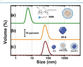
**Figure 1.** Hydrodynamic diameter distribution measured by DLS for: (a) 2 mM DDM solution, which yields monodisperse micelles; (b) ZIF-8 nanocrystals formed after direct mixing of precursors; and (c) ZIF-8 nanocrystals colloidal suspension obtained in (b) with 2 mM DDM solution. For each plot, a schematic illustration of the system obtained is also presented.
