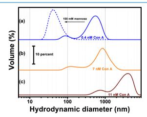
**Figure 2.** Hydrodynamic diameter distribution measured by DLS of Glyco-ZIF-8/Con A supraparticles for different lectin final concentrations: (a) 0.4 nM Con A (solid line –), 0.4 nM Con A added after addition of 100 nM D-mannose (dashed line --), (b) 7 nM Con A, and (c) 11 nM Con A.
