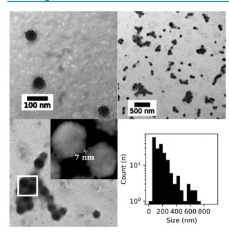
**Figure 4.** (Top) TEM images of Glyco-MOFs before (left) and after (right) 7 nM Con A addition. (Bottom) Distance between two Glyco-ZIF-8 nanocrystals in the presence of Con A (left), and size distribution (right) for the same experiment (7 nM Con A) calculated using the longest distance between any two points on the supraparticle.
