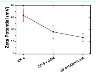
**Figure 3.**  $\zeta$  potential measurements of ZIF-8, Glyco-ZIF-8 prepared with DDM, and Glyco-ZIF-8/Con A supraparticles with a final Con A concentration of 0.4 nM.
