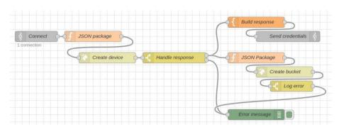
Fig. 2 - Node registration implementation in Node-RED.
