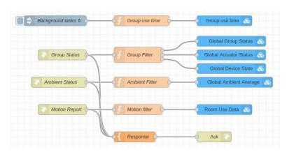
Fig. 3 - Data processing implementation in Node-RED.
