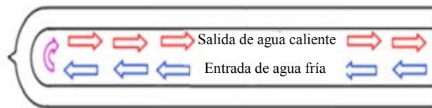
Figura 3: Tecnología del sistema water-in-glass
