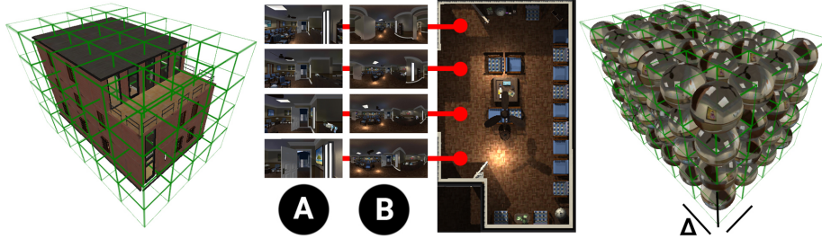
Fig. 3. Image capture example. For each specified camera position, the application captures a 360° panoramic screenshot. (Left) The whole virtual environment is sampled. (Center) Column A shows the camera current view. Column B shows the 360° picture captured at that position. (Right) All the environment is sampled and an image corresponding to each cell of an abstract 3D matrix is generated.
