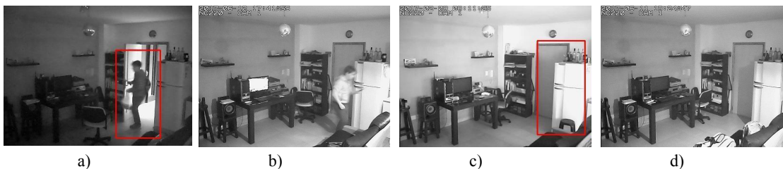
Figure 4. a) True Positive sample; b) False Negative sample; c) False Positive sample; d) True Negative sample
