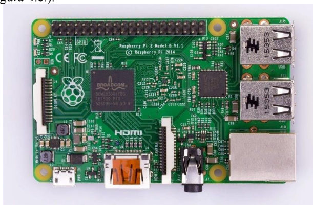
Figura 3. Raspberry Pi 2 modelo B [6].
