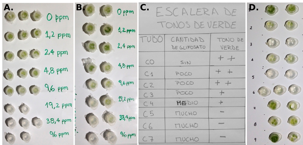
Fig. 8. Example results of typical field assay. A and B. Calibration curves from two different workshops. Numbers in figure indicate glyphosate concentration in ppm (notice comma is used as decimal separator). C. Discussion of glyphosate calibration curve. Sin : without, poco : low, medio : medium, mucho : high, tono de verde : greening. D: Example results of samples assessment.
