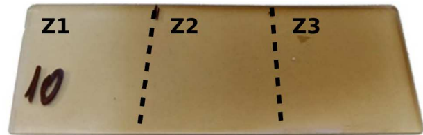
Figure 1. Image of ZnO coatings onto the substrate with three zones: Z1, Z2, and Z3
