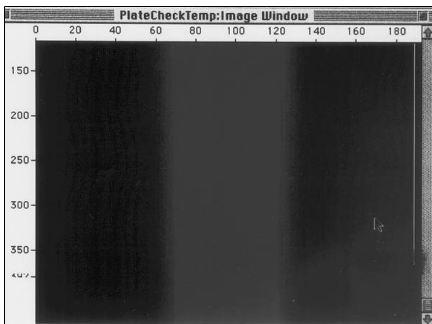
Figure 1. Plate check of an acrylamide “gel sandwich” with both glass plates. Before CeO treatment, the profile of a sequencing gel in the Model 377 DNA sequencer shows a background “green smear”. The x-axis is a measurement of the “channels” (or 194 data points collected by sensors along the sequencing plate from side to side by the CCD-camera) and the y-axis represents arbitrary “ABI fluorescence units”.
