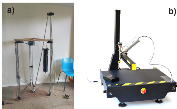
Figure 12: Images of delta printer with an auger extruder printhead (a) [29], and Lutum 3D printer (b) [39].
