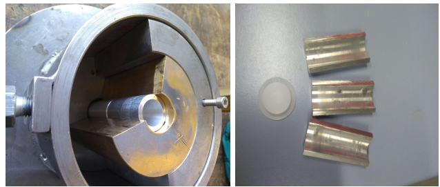
Figure 2. Left panel: Steel housing. Right panel: Aluminium holder with plastic base. The inner diameter of the holder is 1.6 cm.
