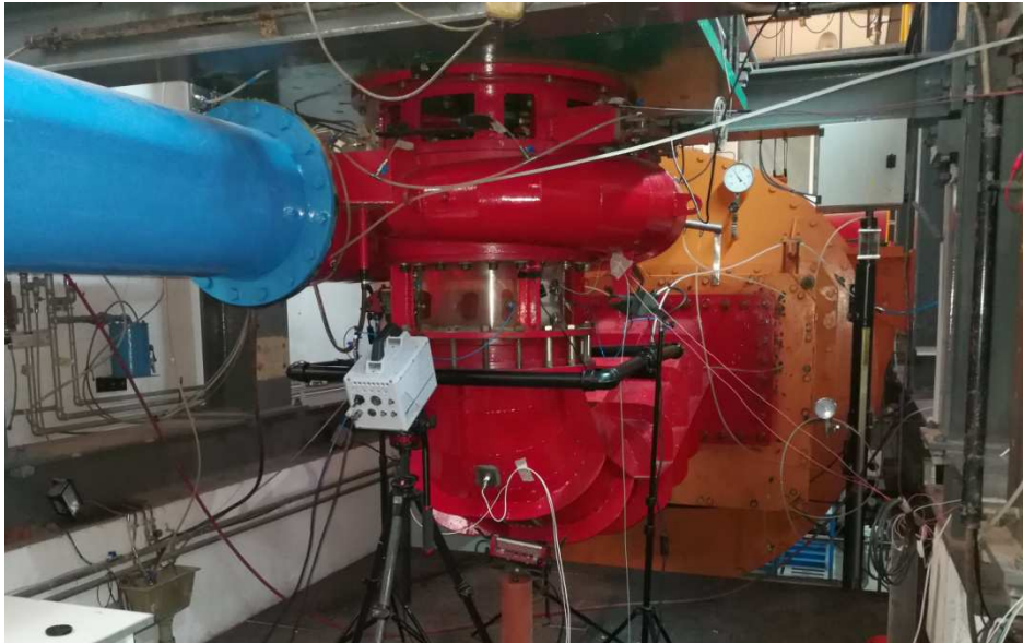
Figure 1. Francis model mounted on the UNLP Test Rig –Laboratory of Hydromechanics.
