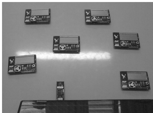
Fig. 4. Implementation of probabilistic query routing using RZRAVEN sensor nodes.
