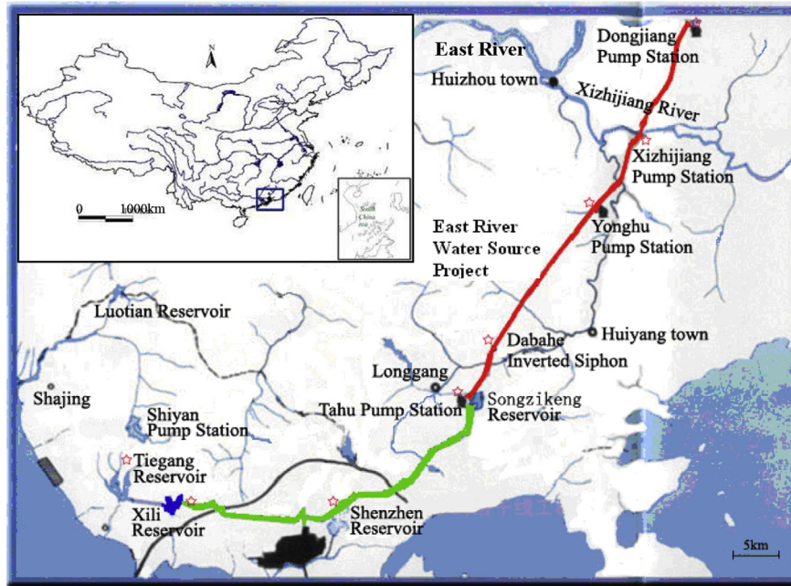
Fig. 1. Layout of the tunnels of East River Water Source Project: red line – water transfer tunnels, green line – water deliver tunnels. (For interpretation of the references to colour in this figure legend, the reader is referred to the web version of this article.)
