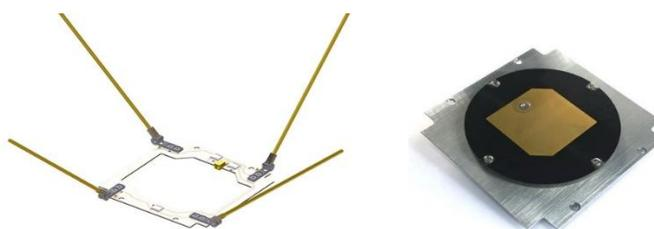
Figuras 2. Antena turnstile      Figura 3. Antena parche
