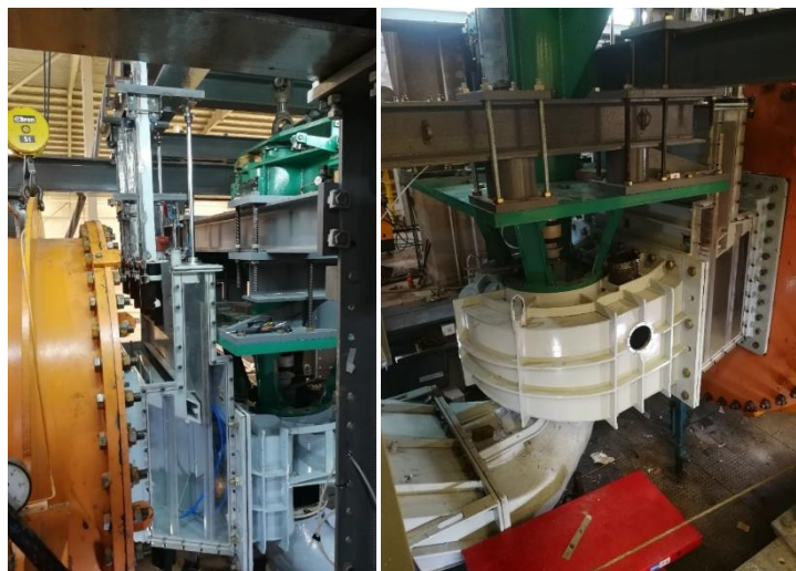
Figure 4. Intake with emergency gates of a Kaplan turbine as mounted on the test rig.
