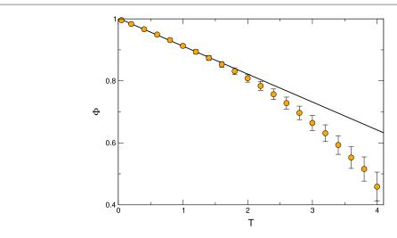
**Figure 6. Polarization.** We report here the polarization in the topological Vicsek model in d = 3 as a function of the temperature (results for the ISM and for metric interaction are identical). The full line is the spin-wave prediction (106).
