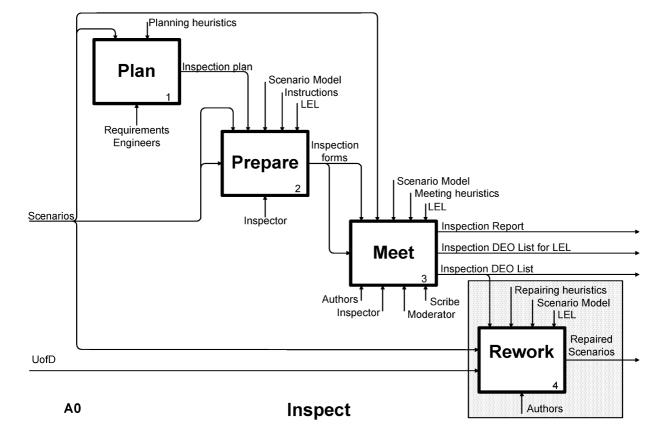
Fig. 7 SADT of our inspection process
