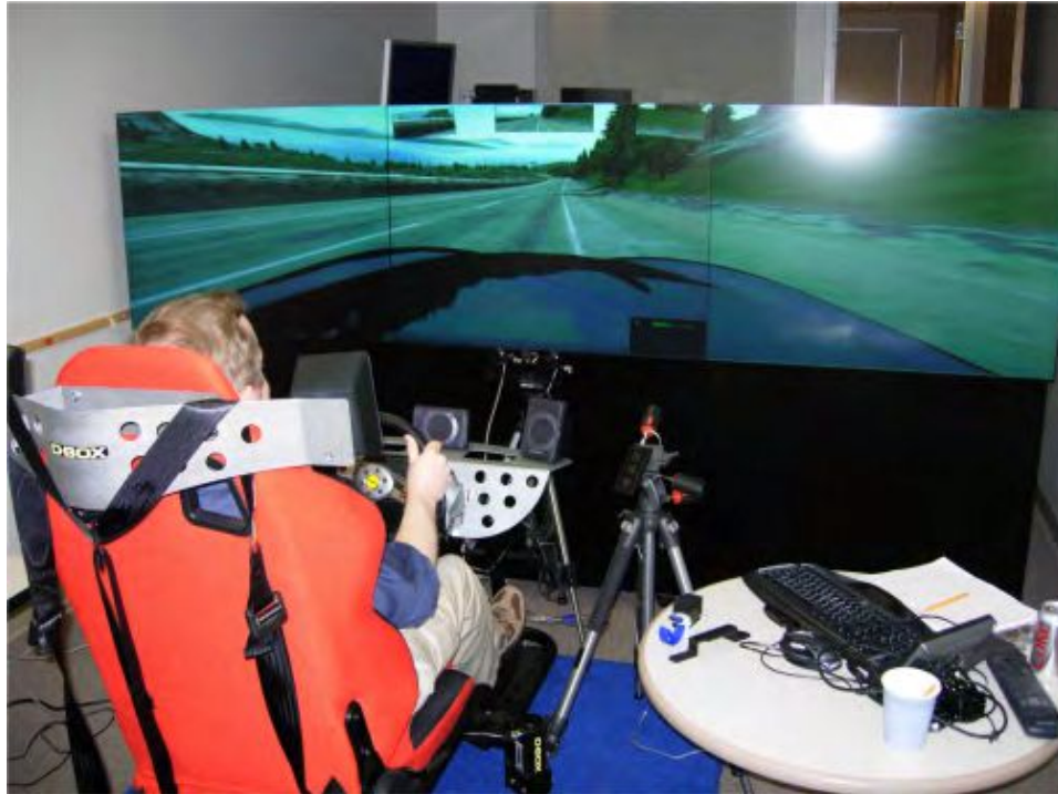
Figura 2.6: Low-Cost driving simulator configuration. Fuente: [11]
