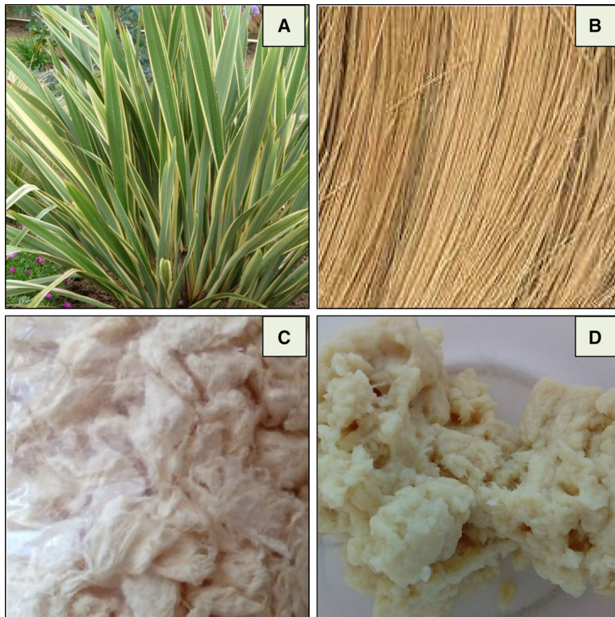
Fig. 1 Phormium ( Phormium tenax ) plant (a), untreated phormium fibers used in this study (b), alkali treated and bleached fibers (c), and refined fibers (d)
