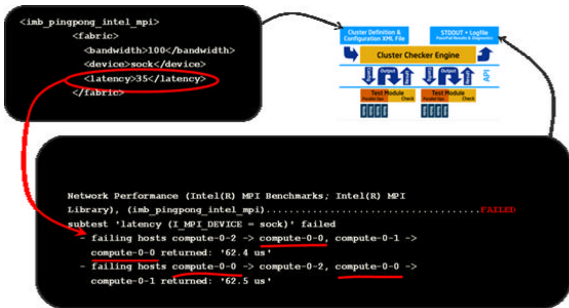
Figure 2c. Test module configuration and result examples.
