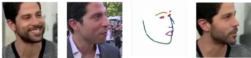
Figure 17: Reenactment scheme. (a) source character image (the one we want to reenact); (b) one of frames of driver actor; (c) extracted facial landmarks that are fed to the reenactment algorithm; (d) reenactment result. 6
