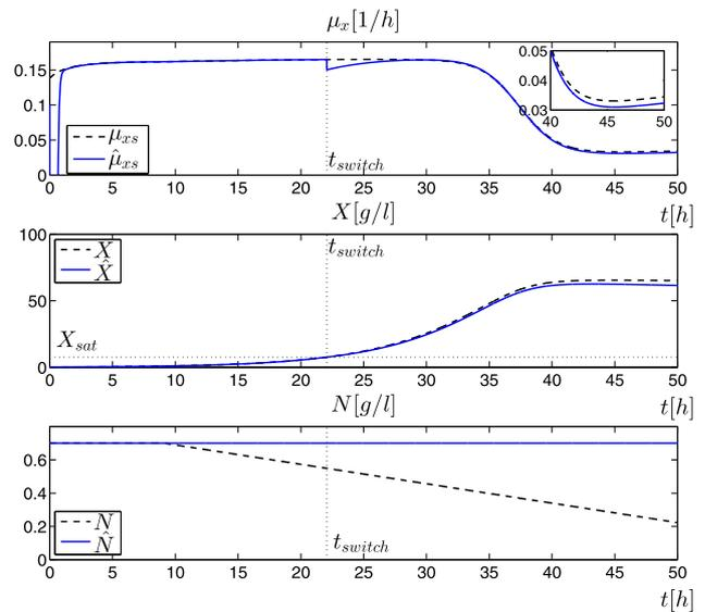
**Fig. 4**  $\mu_{xs}$ -Observer response for a time-varying nitrogen concentration. Simulation results
