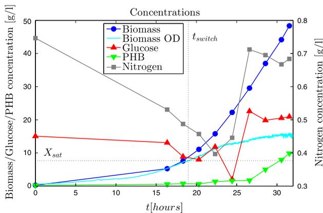
**Fig. 6** Process concentrations. Experimental results. Experiment 1
