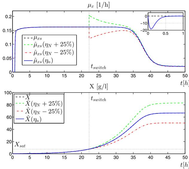
**Fig. 2**  $\mu_{xs}$ -Observer response for different values of  $\eta$ . Simulation results
