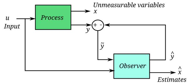
**Fig. 1** Observer scheme,  $u$ : process inputs;  $x$ : unmeasured variables;  $y$ : measured variables;  $\hat{x}$ ,  $\hat{y}$ : estimated variables
