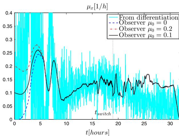
**Fig. 10** Observer response for different initial conditions. Experimental results. Experiment 2
