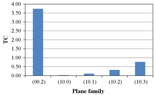
**Fig. 4** Texture coefficient on the flat portion of a washer ( $j = 60 \text{ A/dm}^2$ )
