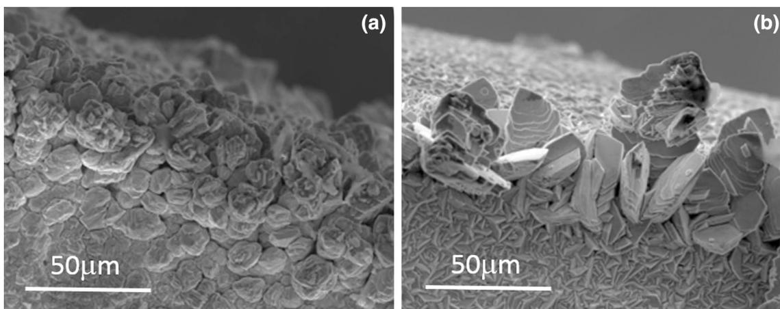
**Fig. 12** SEM micrograph showing dendrite formation at the corner of washer edge: (a) with Na<sup>+</sup> and (b) without Na<sup>+</sup>. Deposits were obtained at 40 A/dm<sup>2</sup> and 800 rpm ( $t = 20$  s)
