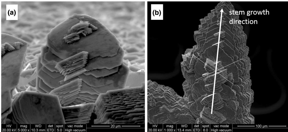
**Fig. 8** SEM micrograph showing the (a) nucleation ( $t = 15$  s) and (b) development of new platelets along a dendrite ( $t = 180$  s)
