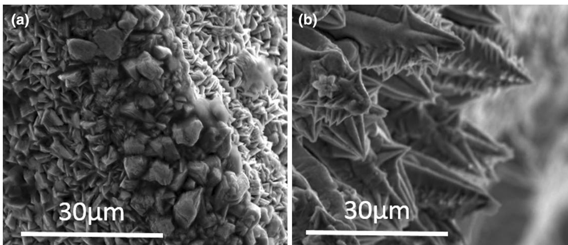
**Fig. 14** SEM micrograph showing dendrite formation at the corner of washer edge: (a) with  $5 \text{ g/L}$  thiourea and (b) without additives. Deposits were obtained at  $60 \text{ A/dm}^2$  and  $800 \text{ rpm}$  ( $t = 5 \text{ s}$ )
