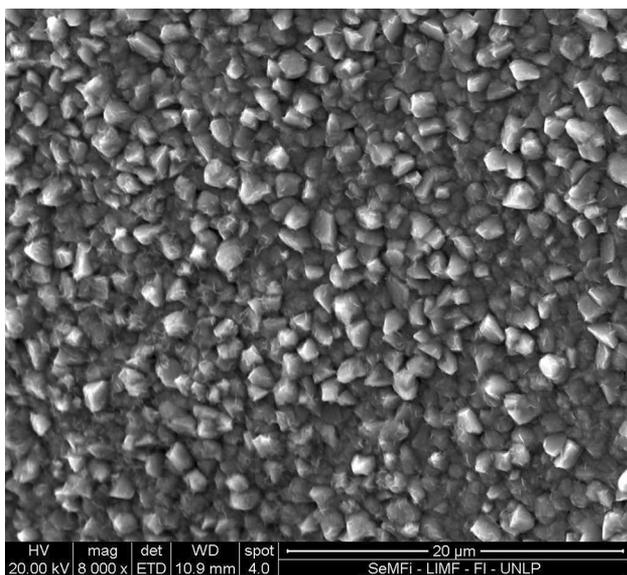
**Fig. 13** SEM micrograph of the flat portion of a Zn deposit obtained in the presence of thiourea ( $5 \text{ g/L}$ ); deposition time  $t = 180 \text{ s}$  ( $j = 60 \text{ A/dm}^2$ )
