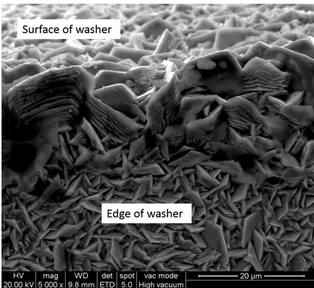
**Fig. 6** SEM micrograph showing dendrite formation at the corner of washer edge; deposition time  $t = 5$  s
