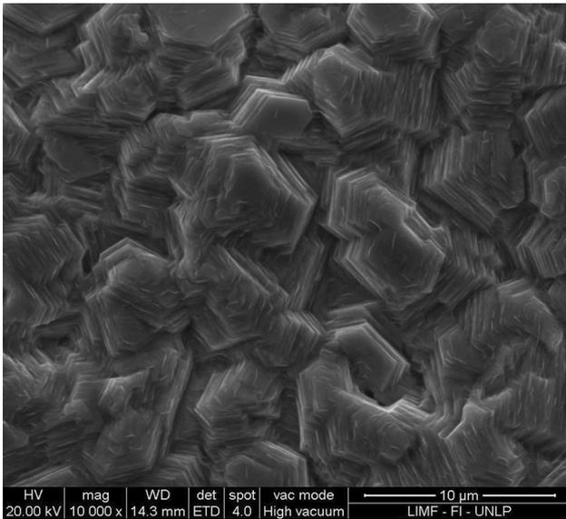
**Fig. 5** SEM micrograph of the flat portion of a washer; deposition time  $t = 180$  s ( $j = 60$  A/dm<sup>2</sup>)
