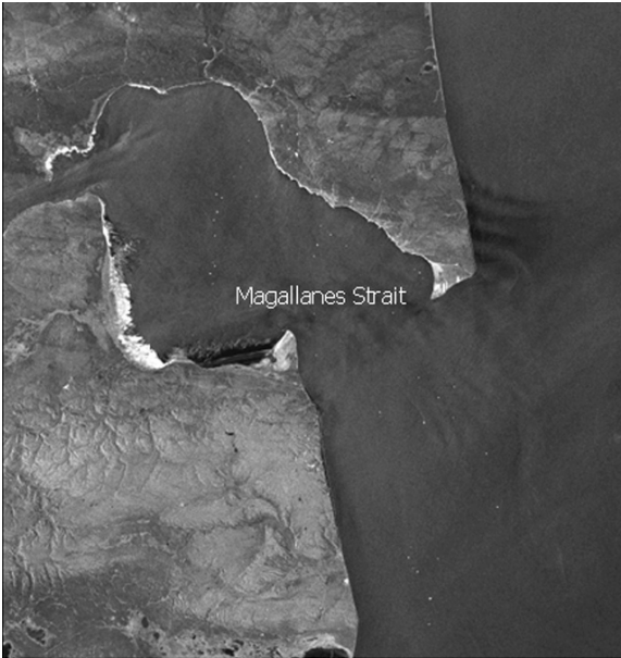
Fig. 12.7 Part of the Radarsat image (Scan Narrow A, May 2004) covering the Magallanes Strait. Note that the bright spots indicate off-shore oil platforms
