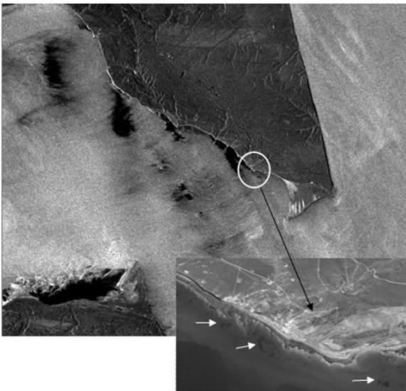
Fig. 12.8 Part of the Radarsat image (Wide 1, Apr. 2007) covering the Magallanes Strait; dark areas are with slow wind and calm water. Part of the QuickBird image (the lower right insert) shows some floating seagrasses, which are indicated with three white arrows
