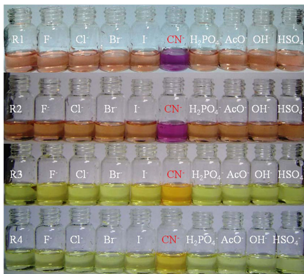
Fig. 11 Colorimetric changes of a R1, b R2, c R3 and d R4 (25 \mu M in 25% aq. DMSO) upon the addition of various anions (1.5 mM in 25% aq. DMSO) [106]
