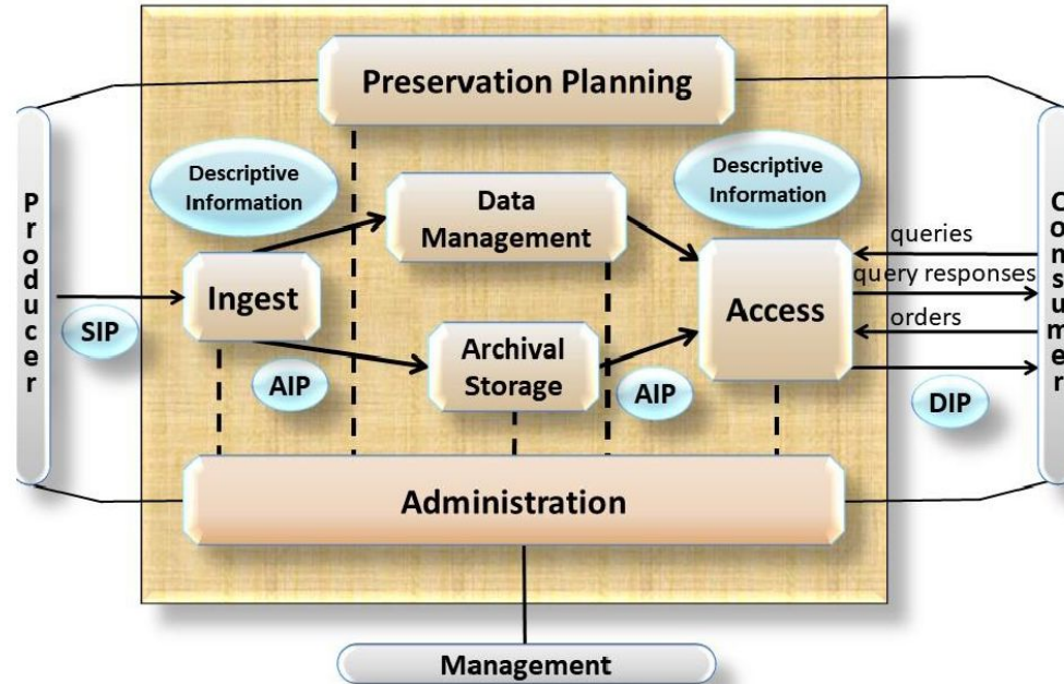
Figure 4-1: OAIS Functional Entities. Management Council of the Consultative Committee for Space Data Systems (CCSDS). (2019). OAIS final v3 draft with changes wrt OAISv2 20190924-rl.docx . P. 41
