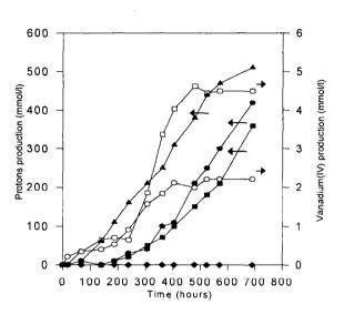
FIGURE 2: Reduction of (V) Vanadium in cultures of Thiobacillus thiooxidans on elemental sulfur. Symbols: Protons (•) and Vanadium(IV) production (O)for initial Vanadium(V) concentration of 2.25 mM; (■),  $(\Box)$  Idem for initial vanadium (V) concentration of 4.50 mM;  $(\spadesuit)$ Idem for initial vanadium (V) concentration of 10.0 mM; ( $\Delta$ ) protons production for the system without vanadium.
