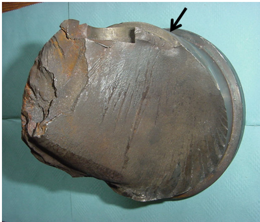
Fig. 2 Generator shaft and coupling with evidence of a torsional fatigue fracture. Craighead and Gray [4] investigation of diesel generator shaft and bearing failures
