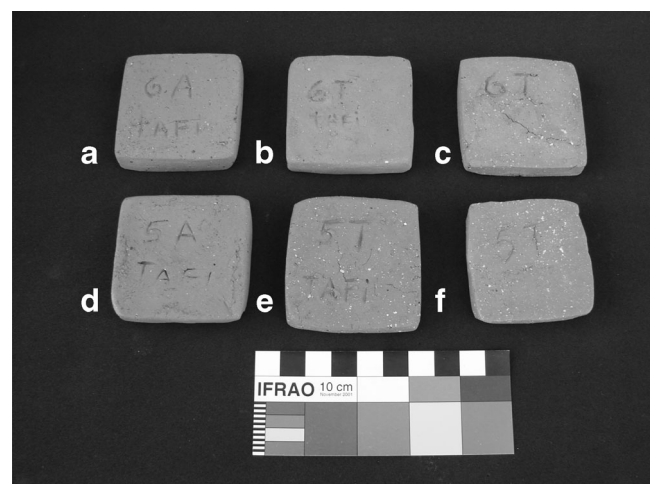
Fig. 4 Briquettes with controlled percentages of inclusions added. a 30 % sand (Tafi); b 30 % pyroclastic inclusions (Tafi); c 30 % pyroclastic inclusions (El Shincal); d 20 % sand (Tafi); e 30 % pyroclastic inclusions (Tafi); f 20 % pyroclastic inclusions (El Shincal)
