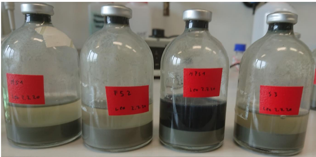
Fig. S12: Serum bottles of abiotic control experiment. One replicate of each treatment, from left to right: slurry + molybdate, slurry + \text{Fe}^{2+} , slurry + \text{Fe}^{2+} + molybdate, slurry only.
