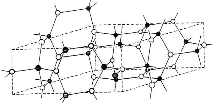
Figure 3. Hexagonal  $\beta$ - $C_3N_4$  lattice, Space Group  $P6_3/m$ .
