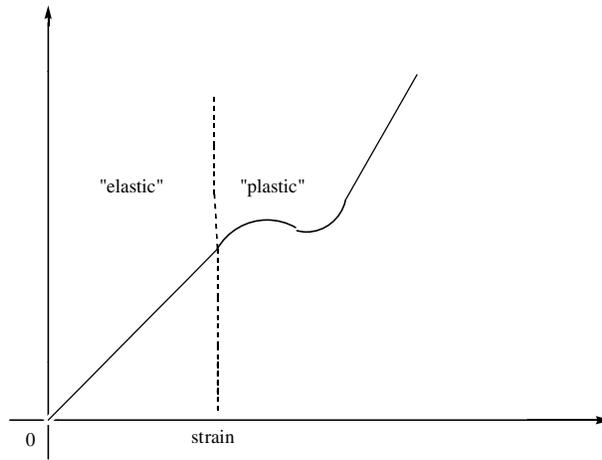
Figure 1. Stress–strain curve for determining moduli of elasticity.
