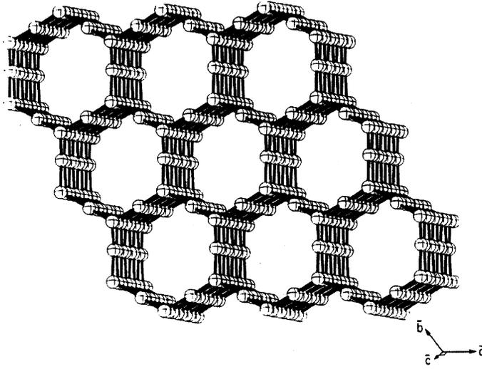
Figure 5. Hexagonal hexagonite lattice, Space Group P6/mmm.
