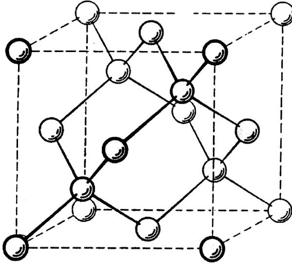
Figure 2. Cubic diamond lattice, Space Group  $Fd\bar{3}m$ .
