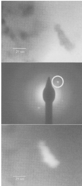
Figure 4. Transmission electron microscopy image of nanoparticles obtained via micro-emulsion. (Top) bright-field image. (Middle) electron diffraction pattern with the spot that gave rise to the dark field image indicated by a circle. (Bottom) dark-field image of the same particle as that at the top.
