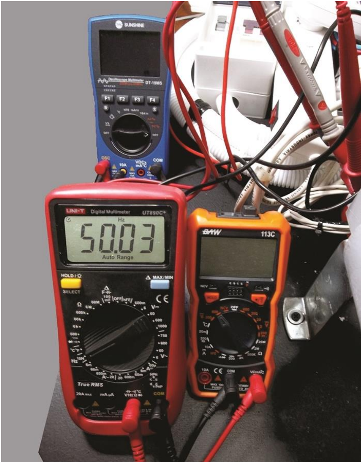
Figure n° 16. View of the frequency meter turned on indicating the 50 (Hertz) of the alternating current (AC), next to the digital multimeter (voltmeter) turned off. Source: Own elaboration.
