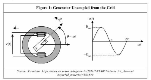
The rotation of the rotor axis causes the flux linked by the stator coil to be variable so that the voltage generated at its terminals is due to the temporary variation of said flux, which is known as the Lenz-Faraday Law:
