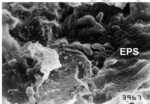
Fig. (6). SEM micrograph showing a sample of 70/30 copper-nickel 7 days after immersion in natural sea water. Bacteria, EPS and corrosion products can be observed (X 3500).
