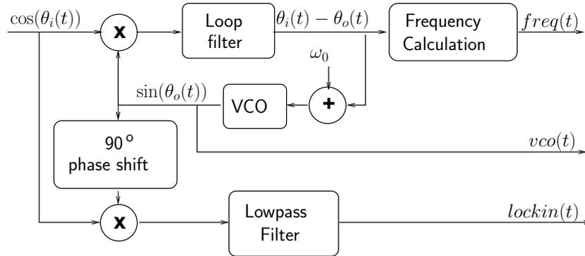
**Fig. 2.** Basic PLL operation.
