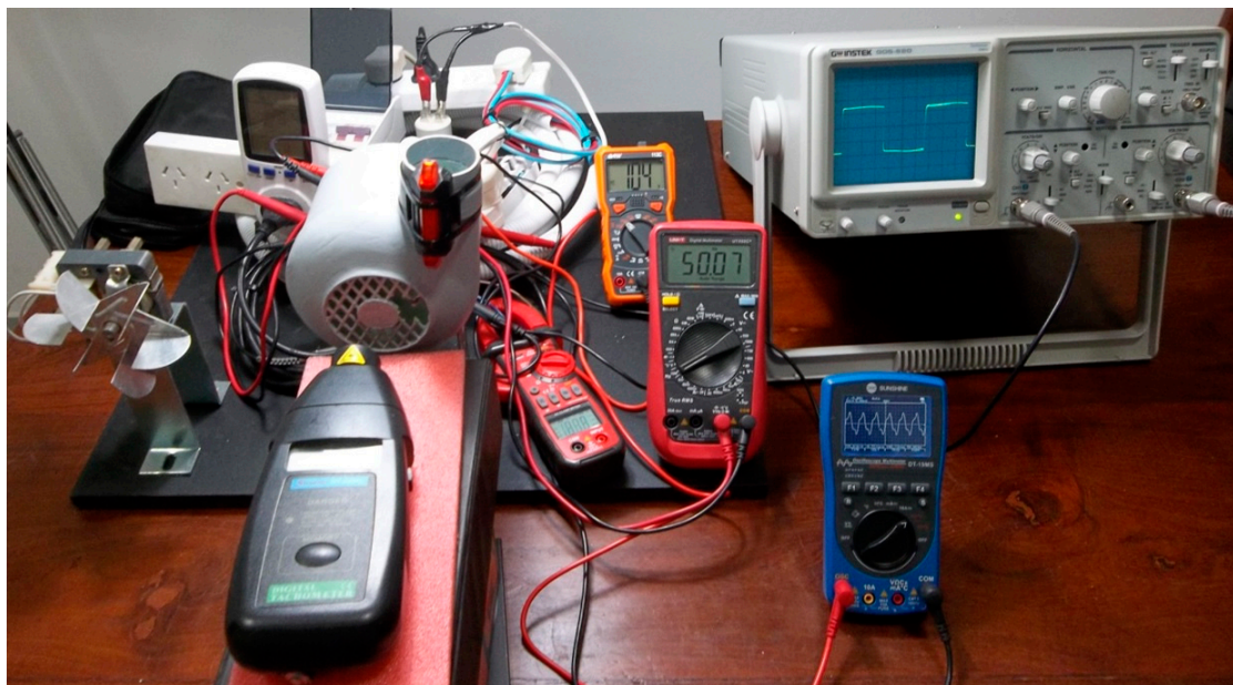
Figure 2. Test bench connected to the PMSM type synchronous motor (as an example). With digital multimeter (volt meter in AC), amperometric clamp (current intensity meter in AC), frequency meter (Hertz meter), laser photocometer (speed meter in RPM), digital oscilloscope waveform meter the alternating current in voltage ( V_{peak} -peak, V_{avg} , V_{rms} ), for calculation of the crest factor of harmonic distortion, analog oscilloscope for qualitative observation of the THD (harmonic distortion of alternating current), wattmeter (active power meter in watts or watts), power factor (cosine of \phi ), power -meter (meter of active energy consumption in kilowatt-hours: kWh). Source: self made.
