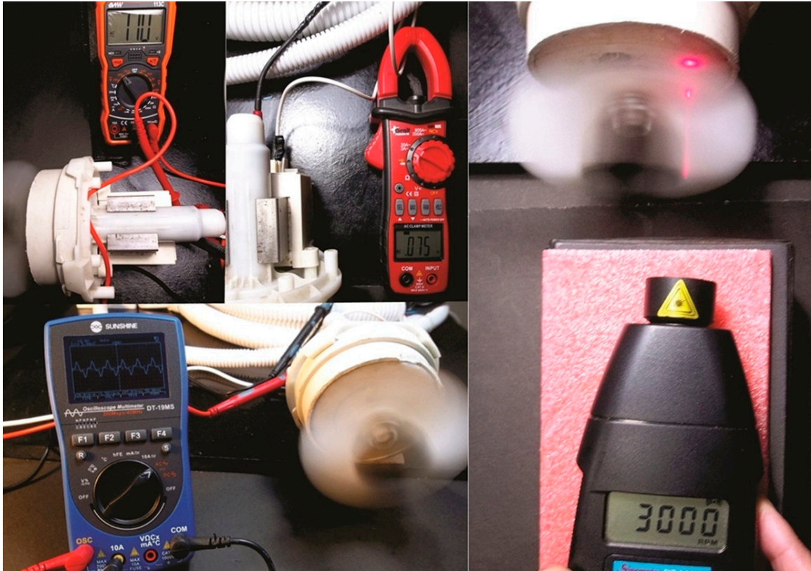
Figure 3. PMSM/IPM type synchronous motor (with the energy efficiency system “on”) connected to the oscilloscope showing the non-linear voltage waveform, also connected to the digital multimeter showing the voltage drop of 110 (Volts), and the amperometric clamp evidencing the drop in the circulation of the electric current at 0.075 (amperes) and the constant in the speed of the blade at 3000 (RPM). Source: self made.
