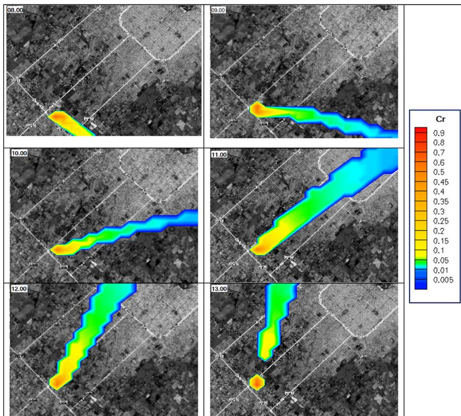
**Fig. 6.** Hourly sequence from 0800 LST to 1300 LST of the modeled smoke plume over the region delimited by the inner rectangle of Fig. 4. The color scale represents the relative concentration of smoke to the source fire computed in all 50-m-side 3-D boxes between the surface and 1200 m. (For interpretation of the references to color in this figure legend, the reader is referred to the Web version of this article.)
