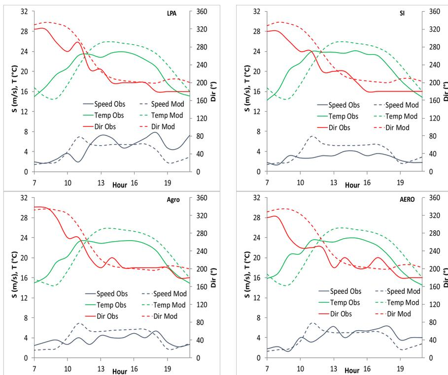
**Fig. 5.** Comparison of BLM forecasts of wind direction (red), wind speed (black) and temperature (green); and observations at La Plata (LPA), Sicardi (SI), Agronomía (Agro) and La Plata Aero (AERO) meteorological stations. Dashed lines correspond to BLM and full lines to observations. (For interpretation of the references to color in this figure legend, the reader is referred to the Web version of this article.)
