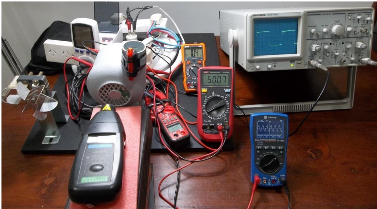
Figure 3: Test bench connected to the PMSM type synchronous motor (as an example). With digital multimeter (volt meter in AC), amperometric clamp (current intensity meter in AC), frequency meter (Hertz meter), laser photocometer (speed meter in RPM), digital oscilloscope waveform meter the alternating current in voltage ( V_{peak-peak} , V_{avg} , V_{rms} ), for calculation of the crest factor of harmonic distortion, analog oscilloscope for qualitative observation of the THD (harmonic distortion of alternating current), wattmeter (active power meter in watts or watts), power factor (cosine of \phi ), power-meter (meter of active energy consumption in kilowatt-hours: kWh). Source: self made.
