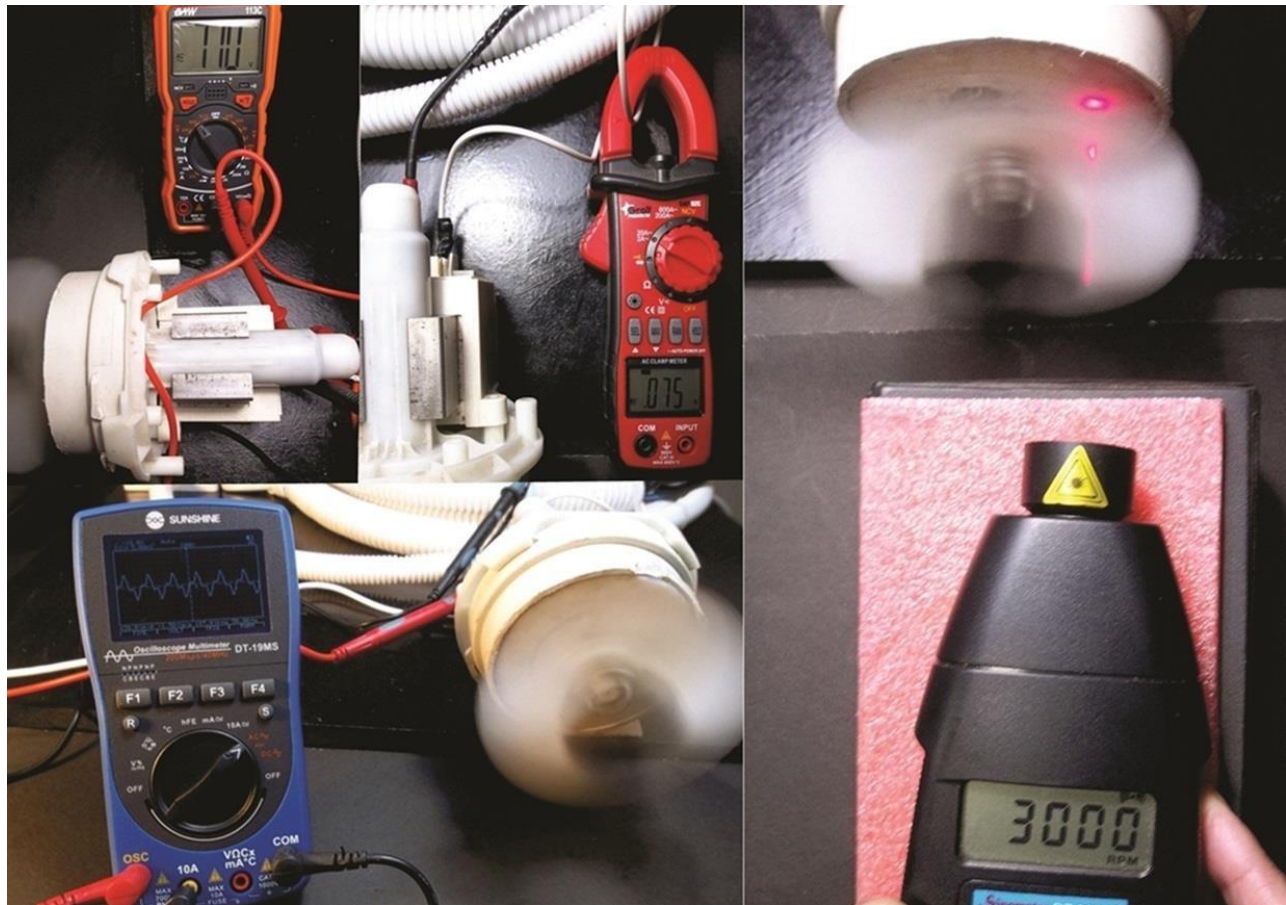
Figure 4: PMSM/IPM type synchronous motor (with the energy efficiency system “on”) connected to the oscilloscope showing the non-linear voltage waveform, also connected to the digital multimeter showing the voltage drop of 110 (Volts) , and the amperometric clamp evidencing the drop in the circulation of the electric current at 0.075 (amperes) and the constant in the speed of the blade at 3000 (RPM). Source: self made.
