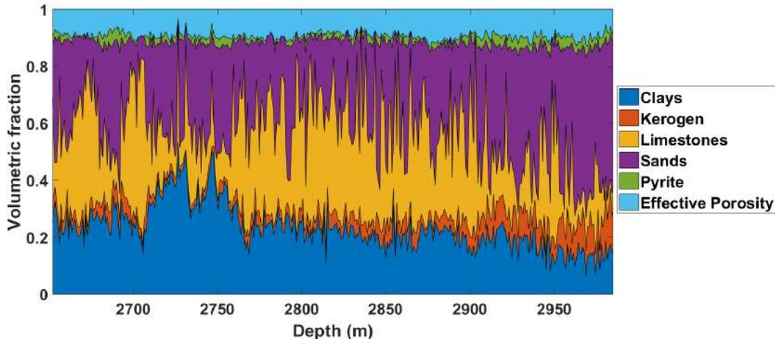
**Figure 1.** Lithological description of VM shale including kerogen fraction and effective porosity.
