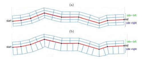
Fig. 8. TT of a river with same parameters (a) and different parametes (b) in both sides
