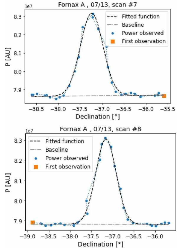
Figure 2: *Upper panel:* Power in arbitrary units (A.U.) for the scan in declination (N-S movement) of Fornax A. *Lower panel:* Power in arbitrary units (A.U.) for the scan in declination (S-N movement) of Fornax A. Both plots show the measurements taken, the fitted function, and the line fitting the baseline. The orange square indicates which observation was made first.
