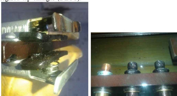
(b) Case 2: high resistance point on the moving and fixed contact of the DETC.
