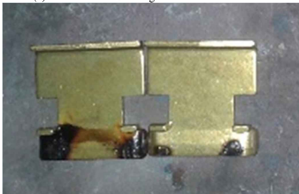
(d) Case 5: high resistance point on the moving contact of the DETC.
