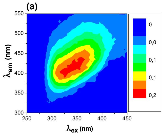
Steady-state excitation – emission matrix of argon-saturated toluene suspensions of BUSiNP inside TOAB micelles.
