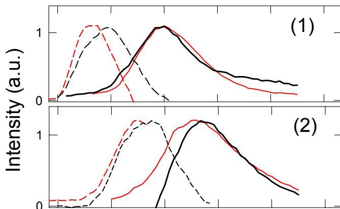
Emission (full lines) and excitation (dashed lines) spectra of species E1 and E2 (graphs **1** and **2**, respectively) contributing to the BUSiNPs excitation-emission matrix, as obtained from the bilinear analysis.
