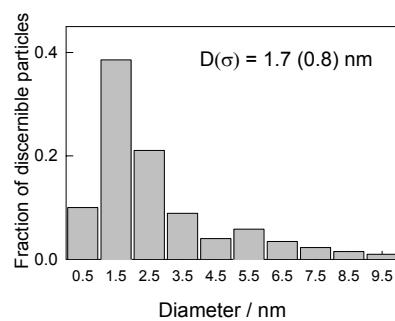
Gaussian distribution is observed with mean diameter of 1.7 nm and 0.8 nm standard deviation.
